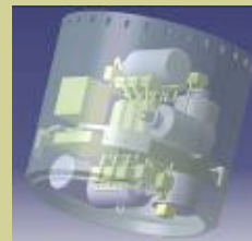
3D view of the EXPLORE setup inside the REXUS experiment module
